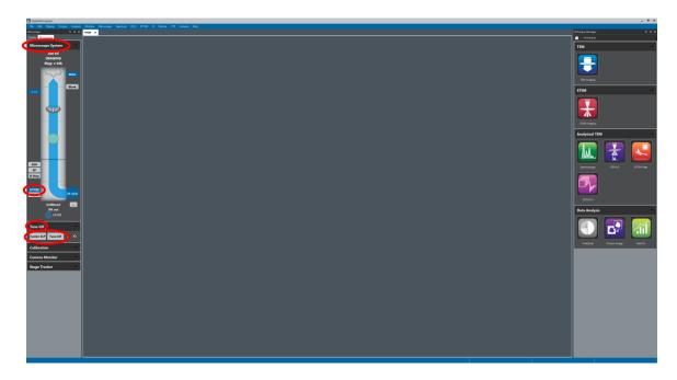
2.7. Re-insert the viewing screen after GIF tuning is complete; no additional GIF tuning should be needed during the session *unless the microscope voltage is changed*.
