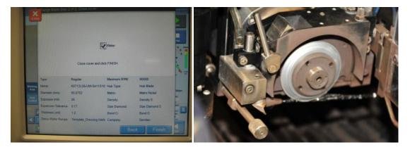
Clean the window and close the door and the spindle enclosure until the lock clicks.
