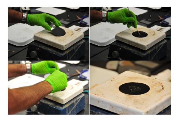
Place the sample very close to the glue pool without toughing it, and drop the sample into the pool face up.
