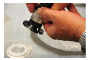
Pull back on the ring to spread the blade flange clamps and gently place the handler on the blade hub flange then release.
