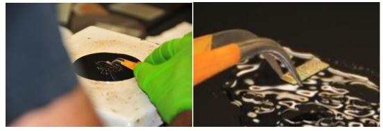
Using a clean swab wooden end gentily press the sample into the pool with a slight circuler motion untill the glue underneath is as thin as possible and the surface of the sample is parallel with the surface of the substrate.
