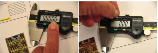
Measure the height and width and record them on the worksheet. One can also at this time "eyeball" measure the dimensions of the individual dies street distances in x and y and record them temporarily. These imprecise measurements can be programmed into the recipe and modified to the precise distances in a later step.
