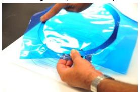
Trim the excess tape from the outside of the ring; make sure that the notches at the top and the flat at the bottom are trimmed flush with the ring.
