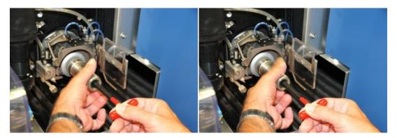
Press the water adjust button and check to see of the jet is aimed at the center of the blade bottom.
