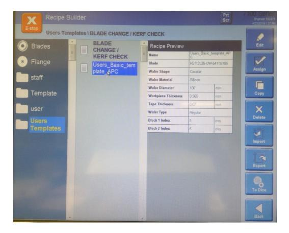
The templates and users templates have most of the basic configurations required already completed. The users templates have been configured more completely to meet our needs; these are the ones users will use.
