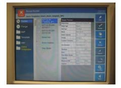
Next click on the "User Templates" menu item and select Blade Change / Kerf Check, then modify the recipe to indicate the assigned blade. Click on the assign button, this will load the Calibration recipe in the machine.
