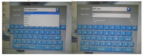
Make sure that the System Init box is checked. Any time the software asks "Do you want to create backup?" the answer will always be yes. The system will proceed through the initialization process, by moving to start position in x,y,z and t. The Main menu should appear.
