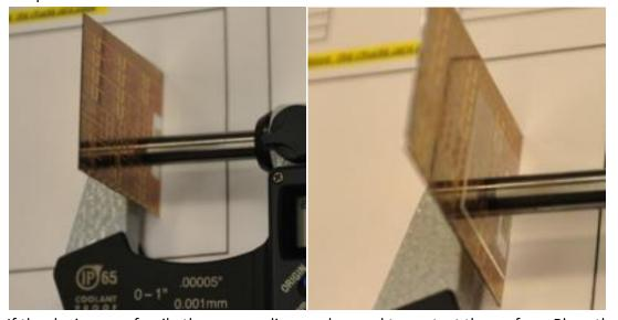
If the devices are fragile then cover slips can be used to protect the surface. Place the protective covers on both sides of the sample and close the jaws, zero the micrometer, loosen the jaws and remove the sample then close the jaws on the covers. This subtractive measurement will be the thickness of the sample.
