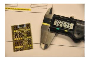
Close the jaws, zero the caliper and select the desired units
