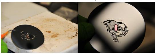
Clean any residual glue off the back with acetone. Measure and record the substrate thickness and mount on the ring with tape as outlined above.
