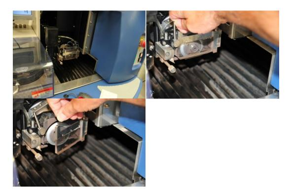
Using the T-handled hex key and the knurled wrench remove the blade retaining nut and place it securely on the black box so that it can't roll away.
