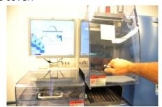
7 Slide the spindle cover latch to the left and...
