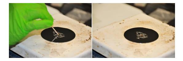
Remove the substrate and allow it to cool, the sample is mounted.
