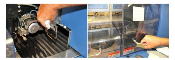
Click the "OK" button then click the finish button; the machine will automatically check and set the blades dimensions using the off the chuck height column. It may warn that the measurements entered are in error, the machine is always right so accept the machines measurements.
