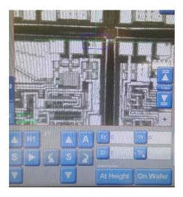
Click finish and then navigate back to the saved position. Center the crosshairs over the area that is to be cut, in this case the middle of the street above the alignment point. Note that the street has a lot of inconsistencies so we will center the cut between the bond pads using the blue box.
