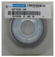
Acquire a new blade from the blade storage drawer and make a post-it label for it using the information printed on the blade. If the blade is a re-load then an "R" would be added to the end of the blade name after the serial number on the existing label.
