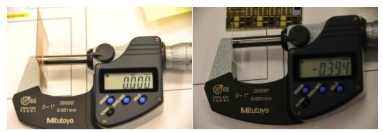
Next, using the calipers (which must be turned on and off manually, by the way) measure the height and width of the sample and record it on the worksheet.
