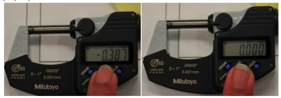
Open the jaws of the micrometer (turn the knurled knob CCW) and place the sample between the post and the rod so that the rod will make contact with the sample in a place that will not damage the devices, close the jaws by turning the knurled knob until it slips.
