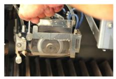
8 open the window so that the blade can be inspected.
