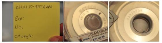
Using a sharp tool score, the security tape on the blade case and carefully open the case
