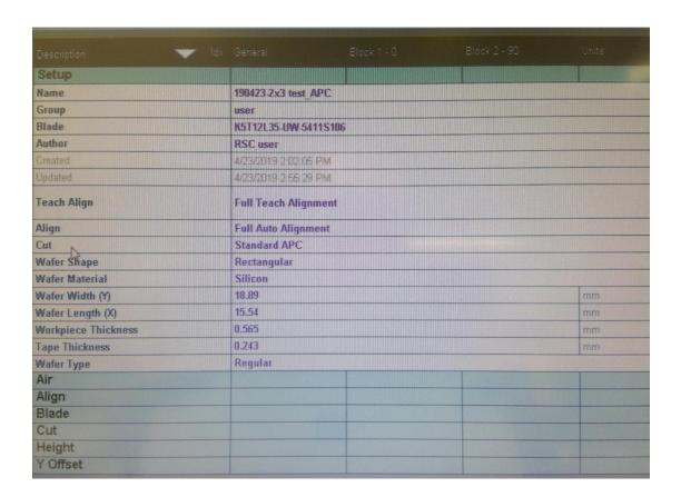
Click save and go on to the Blade section, the air and align sections have nothing that needs to be changed.
