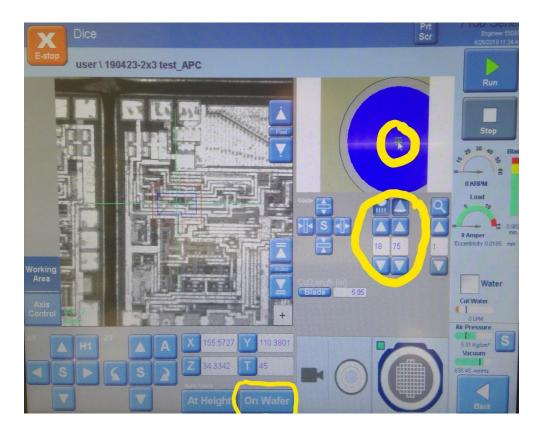
Notice that in the center of the chuck window is an area defined that matches the sample size and shape as designated in the recipe. Double click in the center and the camera will move to the center of the sample. Click the autofocus On Wafer and adjust the illumination control to give a clear video of the sample. The surface of the sample should be in focus, if not there is probably some error in the thickness measurement of the sample stack.
