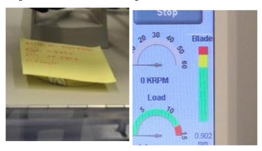
With the above indications it would be advised not to start cutting wafers above 712 um thick as normal blade wear may quickly exceed tolerances.
