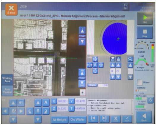
Click next and the will move to the other side of the sample, navigate and place the crosshairs on the identical feature on the left side of the sample.
