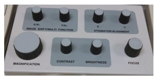
5.10 Focus on the top surface of your sample using the FOCUS and MAGNIFICATION knobs.
