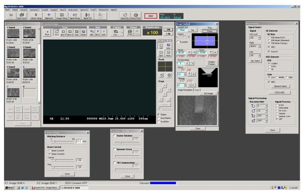
There are operator windows for SCANNING IMAGE, STAGE CONTROL, SIGNAL SETUP, CAPTURED IMAGES, COLUMN SETUP.
