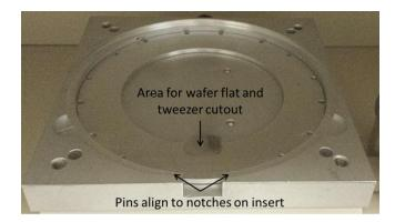
4.3.4. Loading a 2" sample requires the use of all three inserts. Load the 4" insert first, then place the 3" on top, and finally place the 2" insert inside the 3" cutout as shown below.
