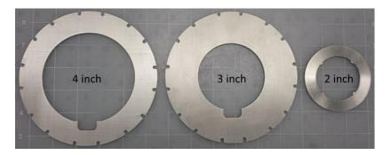
4.3.3. For a 4" or 3" substrate, load the appropriate insert for the diameter of your wafer. There are alignment pins on the stage that the insert will lock into. The wafer flat area should be at the bottom as shown below.
